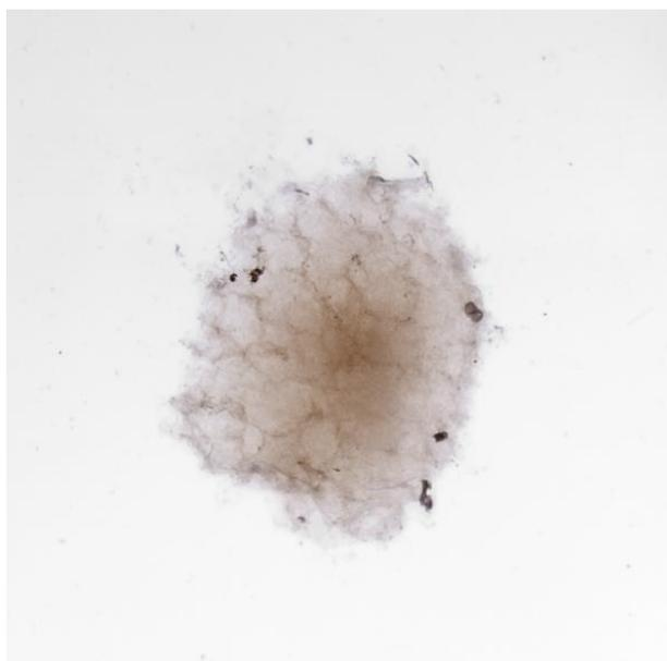
**Fig. 8.** The organized structure in water sample subjected to the temperature +100 °C in the electric field of high voltage and frequency (I. Ignatov, 2014). The material of the electrode – hostafan; the electric voltage – 15 kV, the electric impulse duration – 10  $\mu\text{s}$ ; the electric current frequency – 15 kHz.
