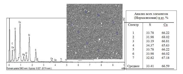
**Fig. 2.** Results of energy-dispersive analysis of Cu₂S film produced by hydrochemical depositin from ammoniac system at temperature 343 K
