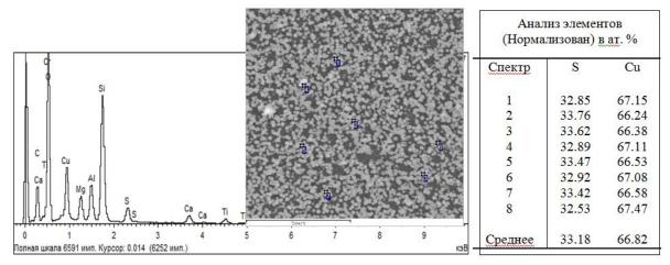
**Fig. 1.** Results of energy-dispersive analysis of Cu<sub>2</sub>S film produced by hydrochemical depositin from acetated system at temperature 298 K
