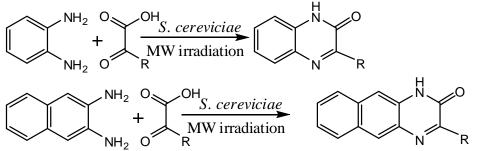
Quinoxalines are effectively synthesized in a few min by the condensation reaction of *o*-phenylenediamine with  $\alpha$ -dicarbonyl compounds in ethanol under microwave irradiation [56]. High yield, short reaction time, pure products without purification and using only ethanol instead of toxic and expensive solvents for isolation of the products, are the advantages of this method.
