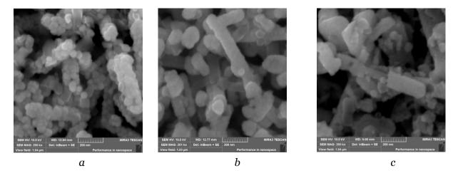
**Fig. 1.** SEM images of as-deposited undoped PbSe thin films (a) and doped PbSe(I) prepared from solution containing NH<sub>4</sub>I mol/L: 0.05 (b); 0.20 (c).
