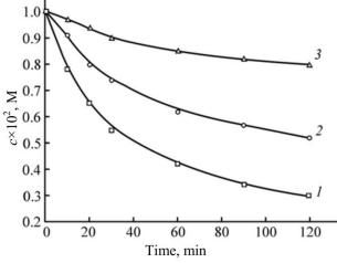
**Fig. 2.** Kinetic curves of the cadmium salt conversion to CdS at (1) 323, (2) 313, and (3) 303 K. Concentrations of the reactants in the reaction mixture, M:  $[CdCl_2] = 0.01$ ,  $[NH_4OH] = 3.0$ ,  $[CS(NH_2)_2] = 0.4$ .
