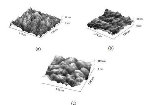
**Fig. 6.** AFM images of the cadmium sulfide films deposited for 120 min at 333 K from the reaction mixture with the concentrations of the reactants, M: (a)  $[CdCl_2] = 0.02$ ,  $[Na_3Cit] = 0.3$ ,  $[CSN_2H_4] = 0.4$ , (b)  $[CdCl_2] = 0.02$ ,  $[NH_4OH] = 2.0$ ,  $[CSN_2H_4] = 0.4$ , and (c)  $[CdCl_2] = 0.02$ ,  $[Na_3Cit] = 0.3$ ,  $[NH_4OH] = 2.0$ ,  $[CSN_2H_4] = 0.4$ , and (c)  $[CdCl_2] = 0.02$ ,  $[Na_3Cit] = 0.3$ ,  $[NH_4OH] = 2.0$ ,  $[CSN_2H_4] = 0.4$  (Scan size 1 × 1 µm).
