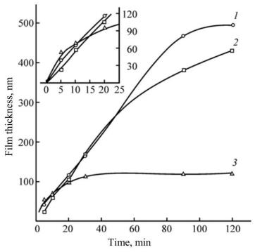
**Fig. 4.** CdS film thickness as a function of the deposition time in (1) ammonia, (2) ammoniacitrate, and (3) citrate systems. Concentrations of the reactants in the reaction mixture, M: [CdCl2] = 0.02, [Na3Cit] = 0.3, [NH4OH] = 2.0, [CSN2H4] = 0.4; T = 333 K; glass-ceramic substrate. The inset shows the initial period of deposition.
