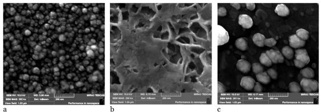
**Fig. 5.** SEM images of the CdS layers and their 3D representations 5 min after the onset of the deposition from (a) citrate, (b) ammonia, and (c) ammonia-citrate systems. Concentrations of reactants in the reaction mixture, M:  $[CdCl_2] = 0.02$ ,  $[Na_3Cit] = 0.3$ ,  $[NH_4OH] = 2.0$ ,  $[CSN_2H_4] = 0.4$ ; T = 333 K.
