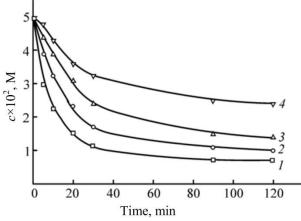
**Fig. 3.** Kinetic curves of the cadmium salt conversion to CdS upon introduction into the reaction mixture of (4) 6 g of classified glass powder and (3–1): (3) 3, (2) 6, and (1) 10 g of the glass powder previously coated with CdS. Concentrations of the reactants in the reaction mixture, M:  $[CdCl_2] = 0.005$ ,  $[NH_4OH] = 3.0$ ,  $[Na_3Cit] = 0.1$ ,  $[CS(NH_2)_2] = 0.4$ ; T = 318 K.
